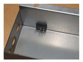
2. Attach the wires to the new switch. The circuit is not polarized so it makes no difference which connector is on top or bottom.
